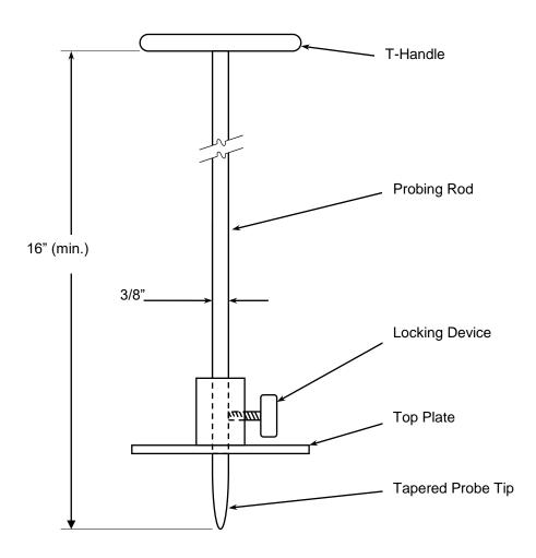
Figure 2.1) Thickness Probe
