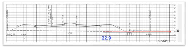
The existing elevation is the *lowest point* across a cross section within a 1:2 control line for a fill section. For cut sections, the existing elevation is the *highest point* within a 1:2 control line. This value is not given. It must be located by selecting the lowest/highest point in the diagram and then scaling to the elevation on the cross section.
