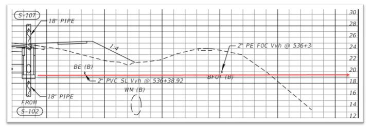
The invert elevation is rarely given on the Plans. If it is not given, then it must be scaled from the Plan cross sections. This drawing does not depict the bottom slab; however, MAC accounts for that. If the structure bottom slab is greater than 8", make note of that for plotting in MAC later.
