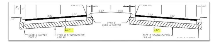
The stabilizing thickness is shown on the typical section diagram. It is almost always 12". Check the typical section to ensure this is the correct thickness.
