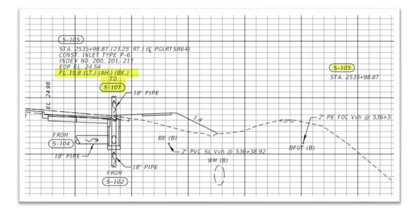
The flow line for each pipe run can be found on the Drainage Structure sheets. This depicts the flowline of S-105 for the pipe run from S-105 to S-107.
