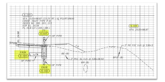
This structure has three other structures connected to it so it would need 3 pipe runs:
