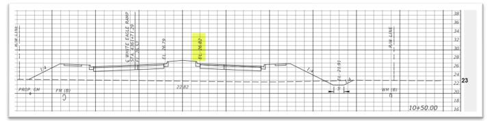
The proposed elevation on a cross section within a 1:2 control line in most cases is given, but if it is not, scale the elevation from the cross section. The value represents the highest proposed elevation of the finished pavement.
