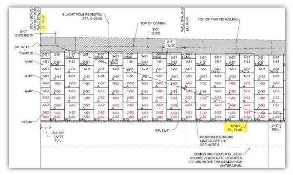
i. Obtain top and bottom elevation from the MSE wall shop drawings.
