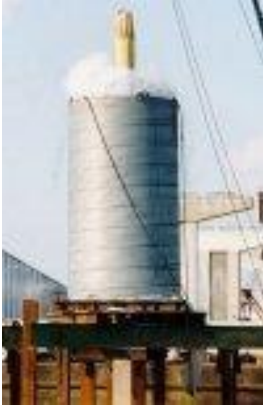
Figure 10-2: Axial Statnamic Load Test
