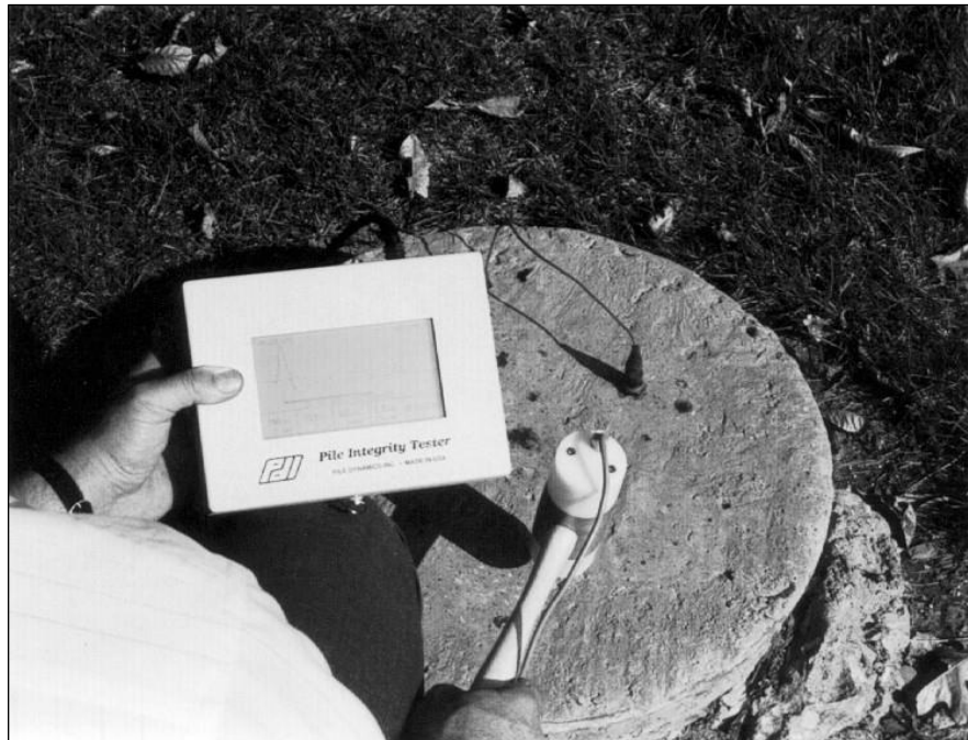
Figure 10-5: Pile Integrity Tester (After PDI, 1993)
