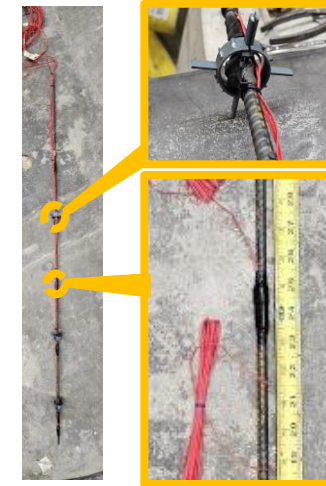
Strain gauge attached to the rebar
