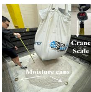
Placement of sandbags and crane scale
