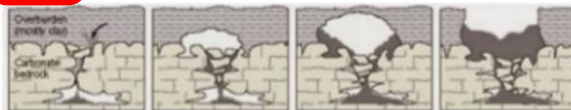
Example: Evolution of Cover-collapse Sinkhole (Soil Arching)
