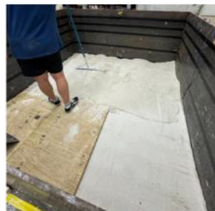
Compacting the sand up to the target level
