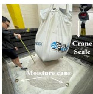
Placement of sandbags and crane scale
