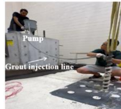
Injection of grout while extracting auger
