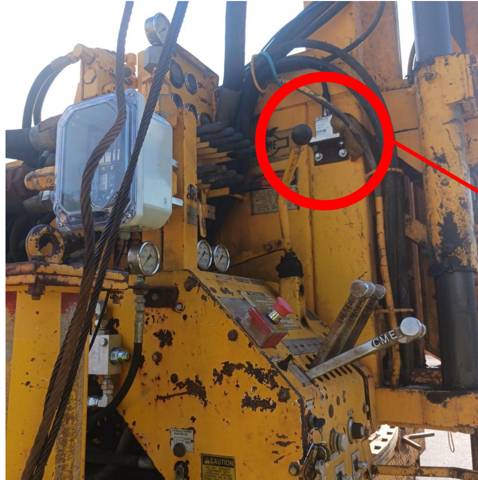
Measure drilling vibrations on the drill rig
