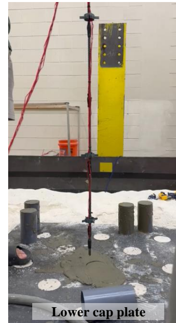
Installation of the strain gauges, cap and loading plates
