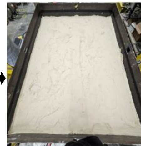
Completion of sand compaction process
