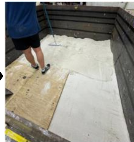
Compacting the sand up to the target level
