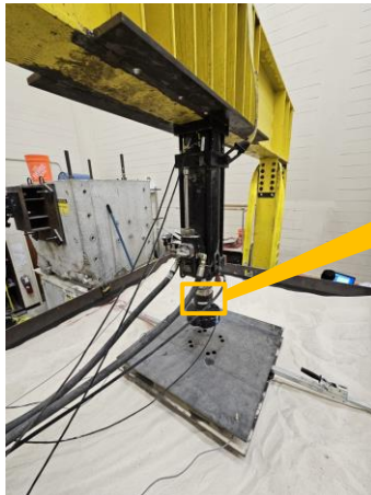
Load cell installed between the actuator and the loading plate
