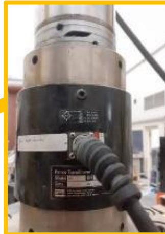
Load cell installed between the actuator and the loading plate
