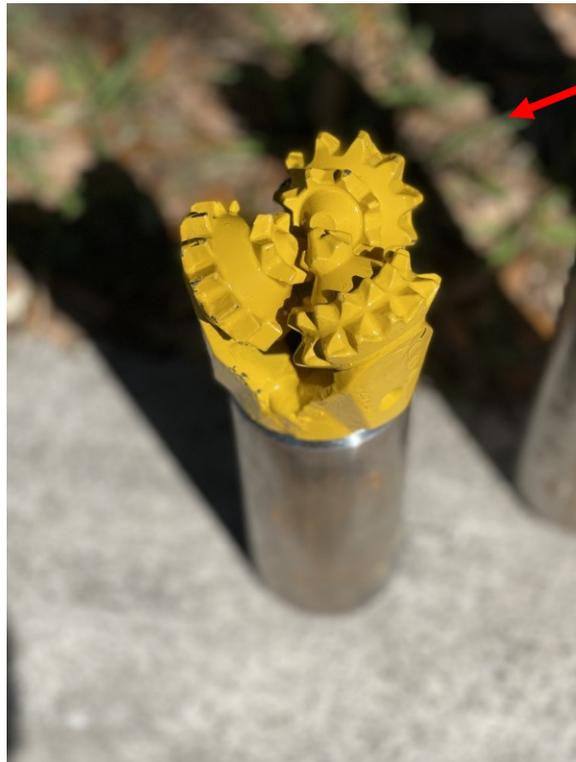
Steel Tooth Tri-cone Roller Bit
