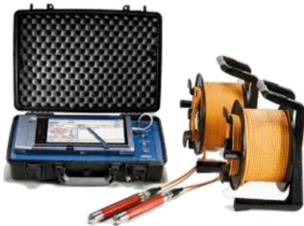
CSL manufactured by Pile-Test.
