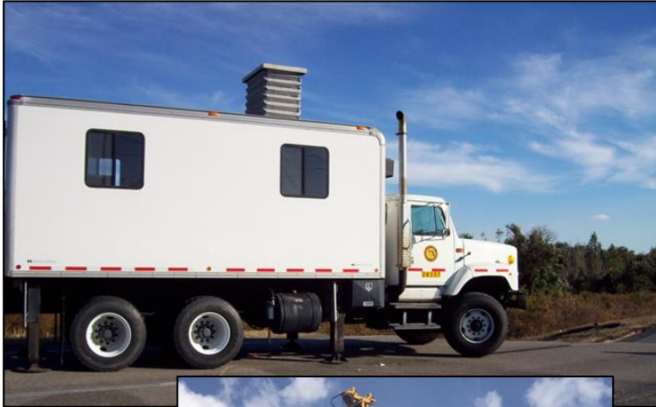
Cone Penetration Test (CPT) SMO team
