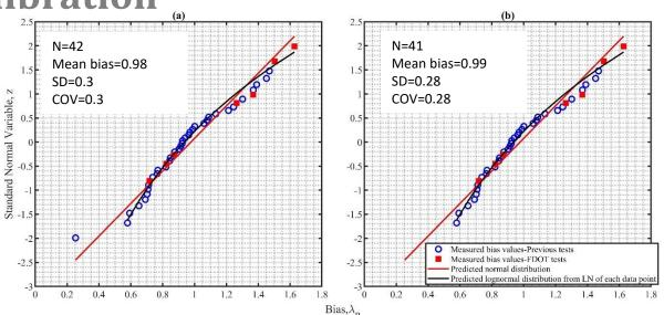
Standard normal variable as a function of bias. (a) Before removing outlier (b) After removing outlier (MP-B test from Adams et al. (2007)).
