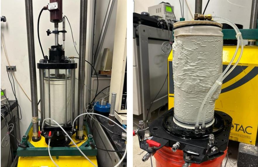
6" diameter triaxial test
