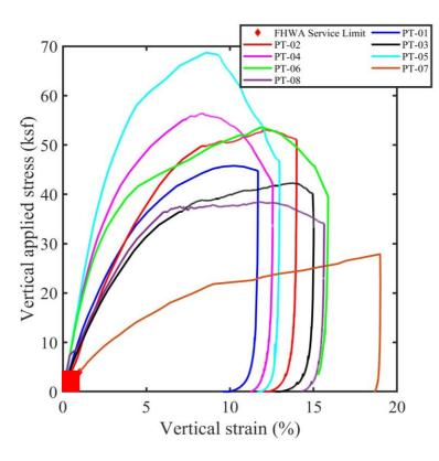
Stress and vertical strain at FHWA service limits
