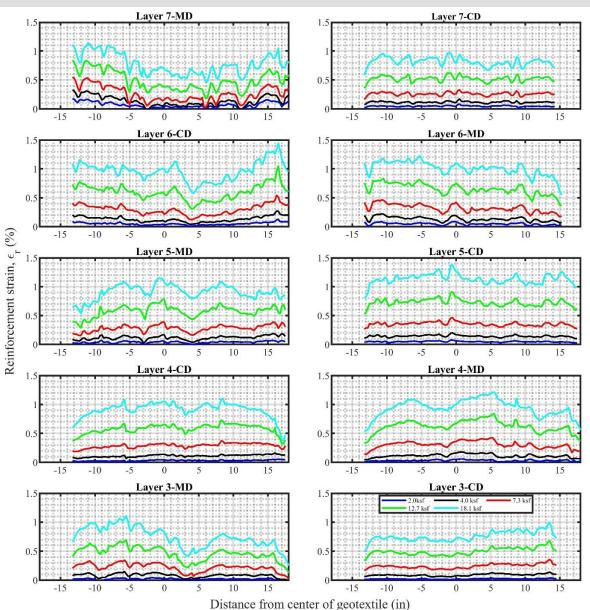
Reinforcement strain distribution in geotextile at different applied vertical stress for PT-05
