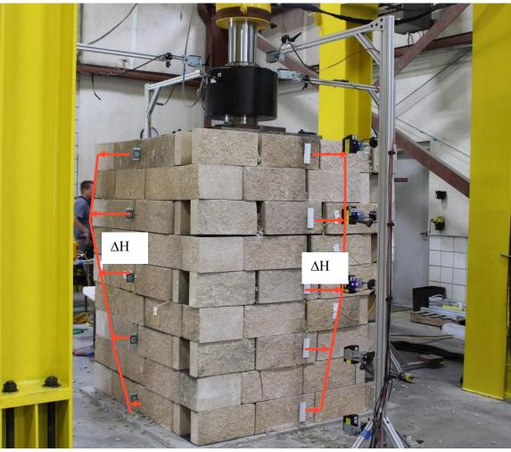
Illustration of lateral displacement after the test
