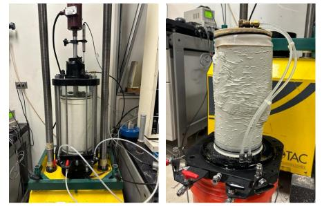
6" diameter triaxial test
