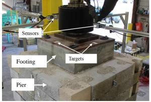
Vertical displacement measurement
