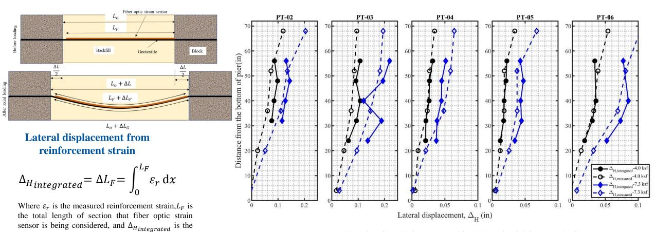
Comparison of lateral displacement estimated from the integration of reinforcement strain with measured lateral displacement at different applied vertical stresses
