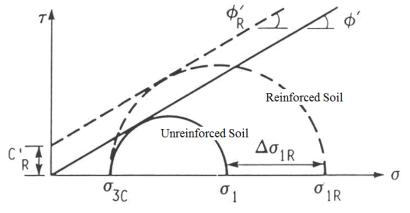
Introduction of apparent cohesion due to reinforcement (Pham, 2009)
