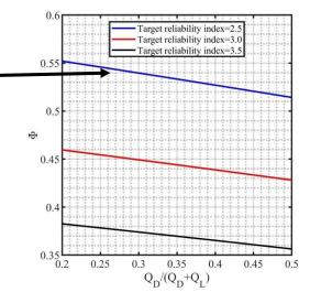
A plot of resistance factors versus dead to dead plus live load ratios for different reliability indices using all data from literature and current study
