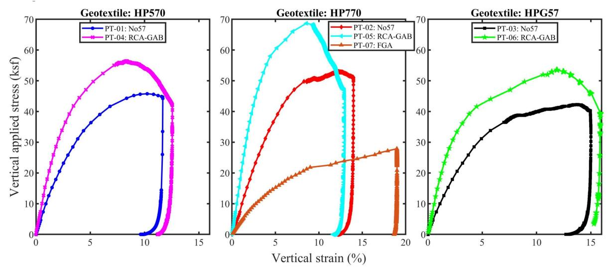
A plot of applied vertical stress versus average vertical strain
