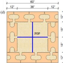
Installation of strain gauges and fiber optic strain sensor **SG**: Strain Gauge; **FOP**: Fiber optic cable
