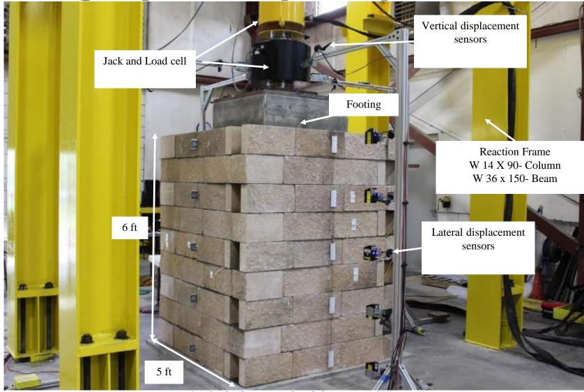
Completed and instrumented pier before testing PT-01
