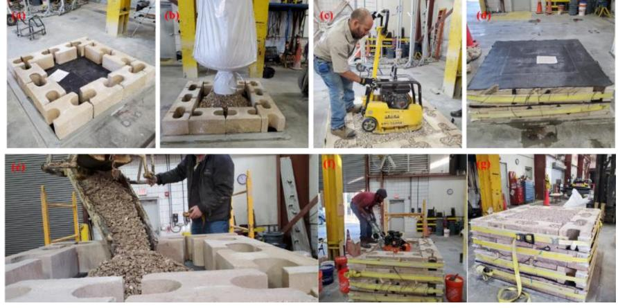
(a) Laying the face blocks, (b and c) Placing and compacting backfill, (d) Laying down geosynthetics, (e, f, and g) Repeat A-C to achieve final height
