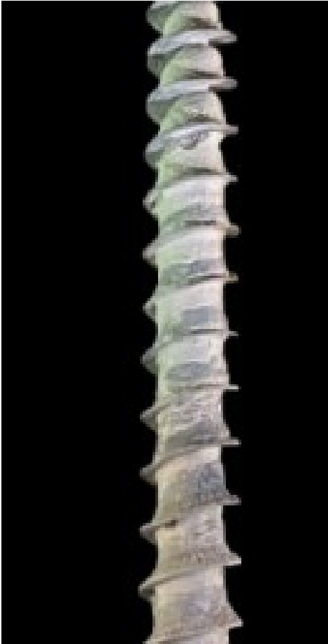
Soil cuttings adhere to auger stem
