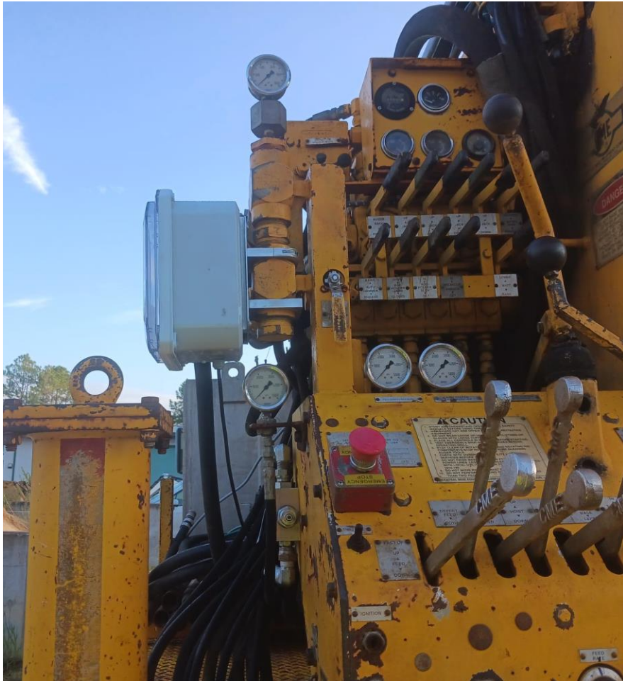
IP68 SBC enclosure for acquiring wireless data
