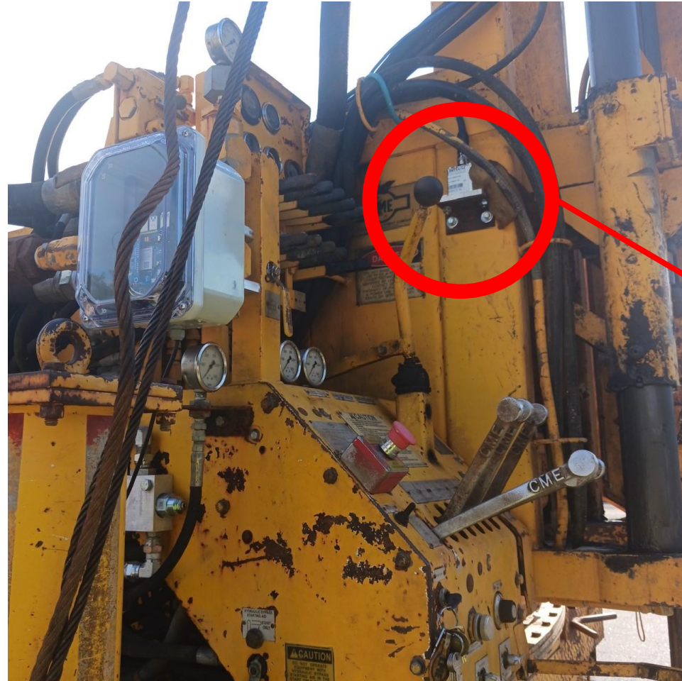
Measure drilling vibrations on the drill rig
