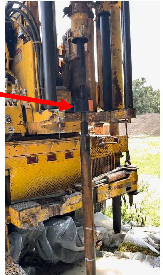
Begins sampling drill rod data after the MWD system is powered on
