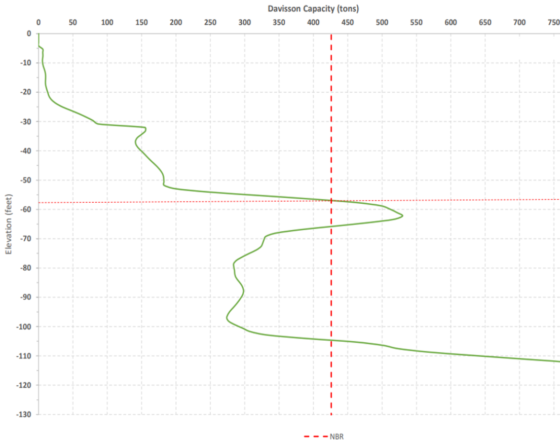
30 Inch - PCP Pile
