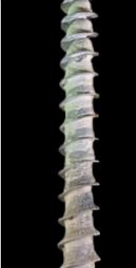
Soil cuttings adhere to auger stem
