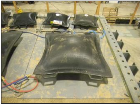
Inflated airbag to simulate overburden pressure (ABOVE)
