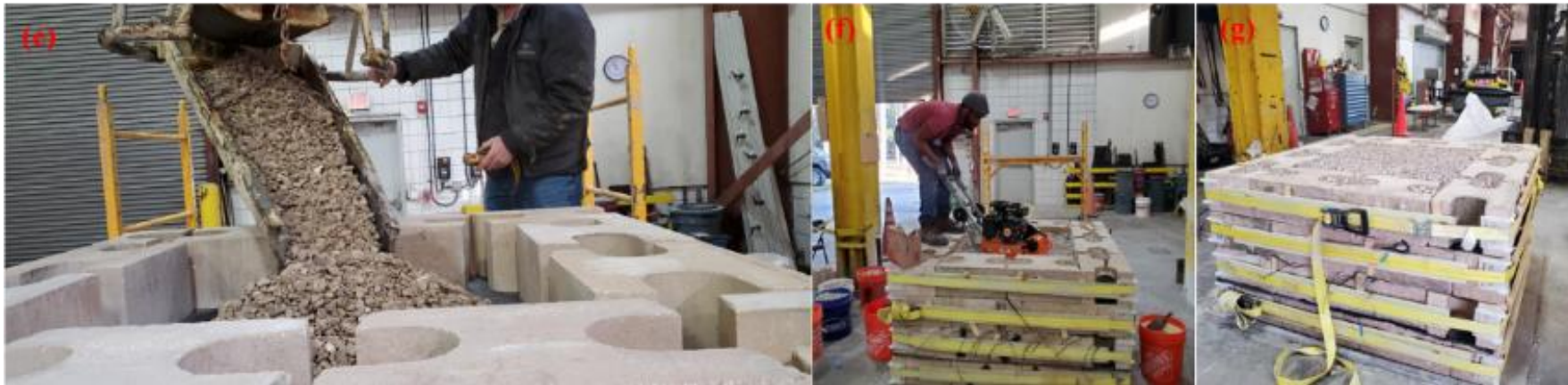
GRS test pier construction steps.
