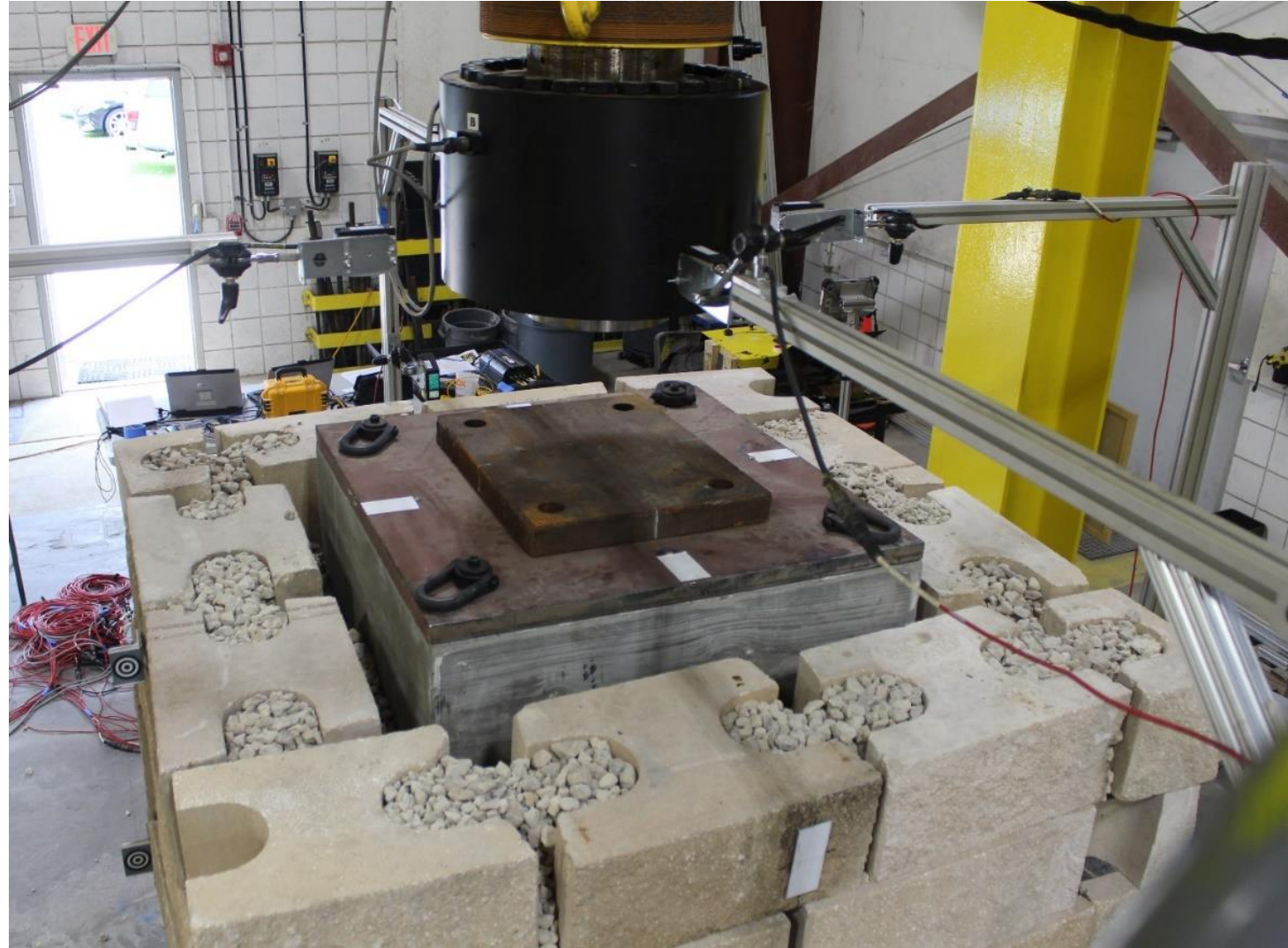
Top view of the failed pier after the PT-01 test
