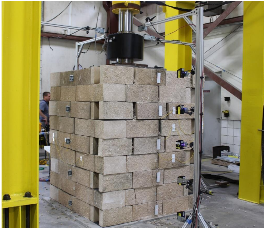
Failed pier after the PT-01 test
