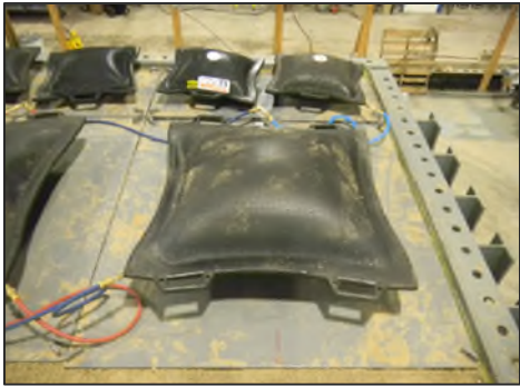
Inflated airbag to simulate overburden pressure (ABOVE)
