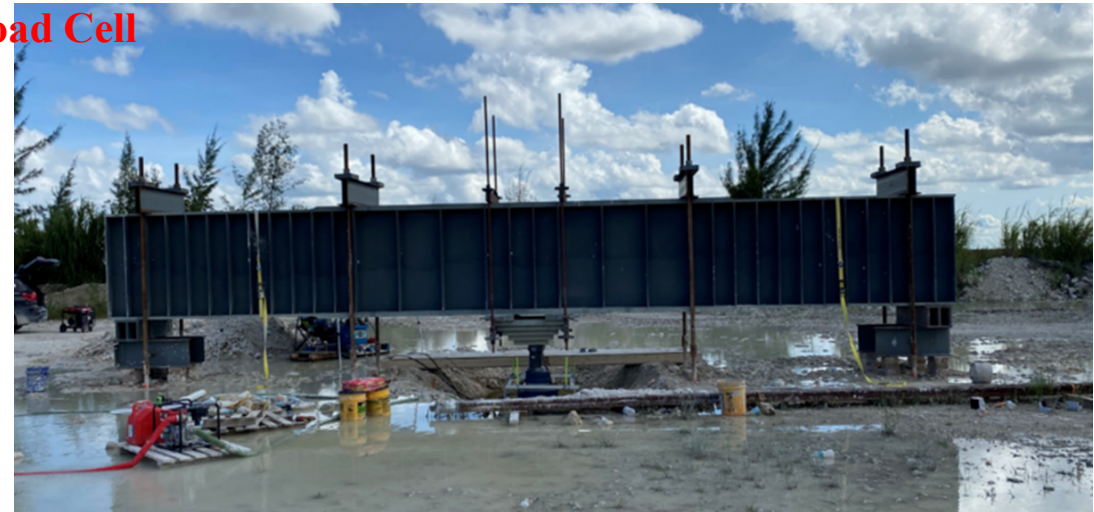
Construction for load test: Anchor Installation, Hydraulic Jack & Load Cell, load test.
