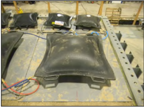
Inflated airbag to simulate overburden pressure (ABOVE)
