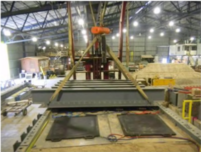
(LEFT) Installation of I-Beam roof for reaction force of airbags and overburden simulation
