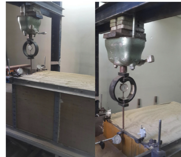
Figure 5: Pictures of the sheet pile under axial loading (Azzam & Elwakil, 2017)
