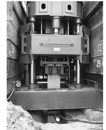
Figure 5: Photos of the test setup for the axial load test (Sylvain et al., 2017)
