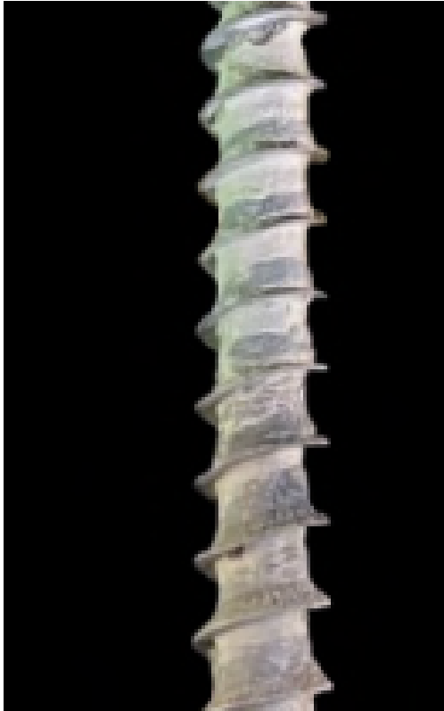
Soil cuttings adhere to auger stem
