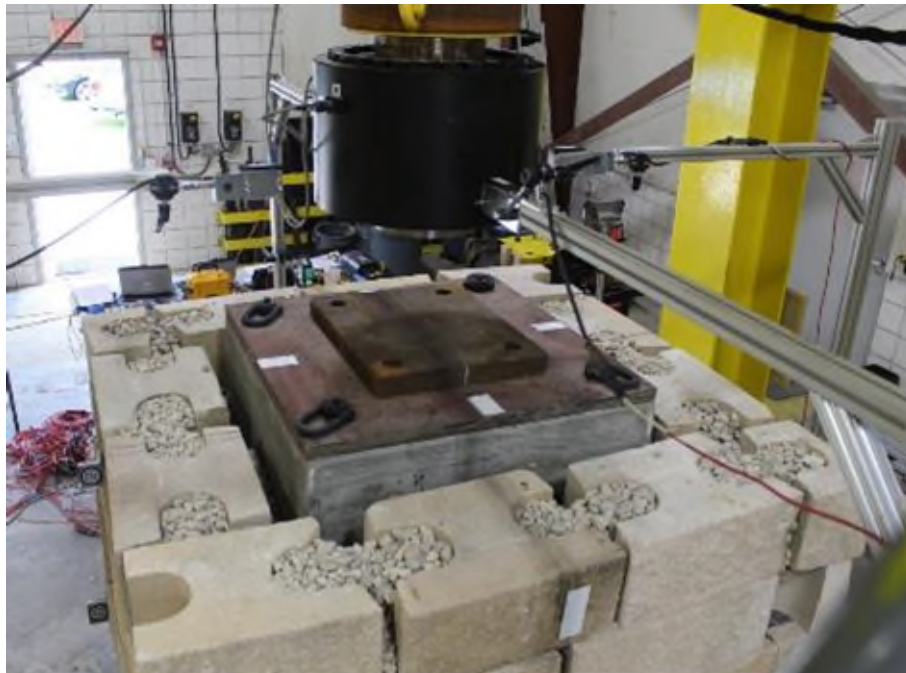
Top view of the failed pier after the test
