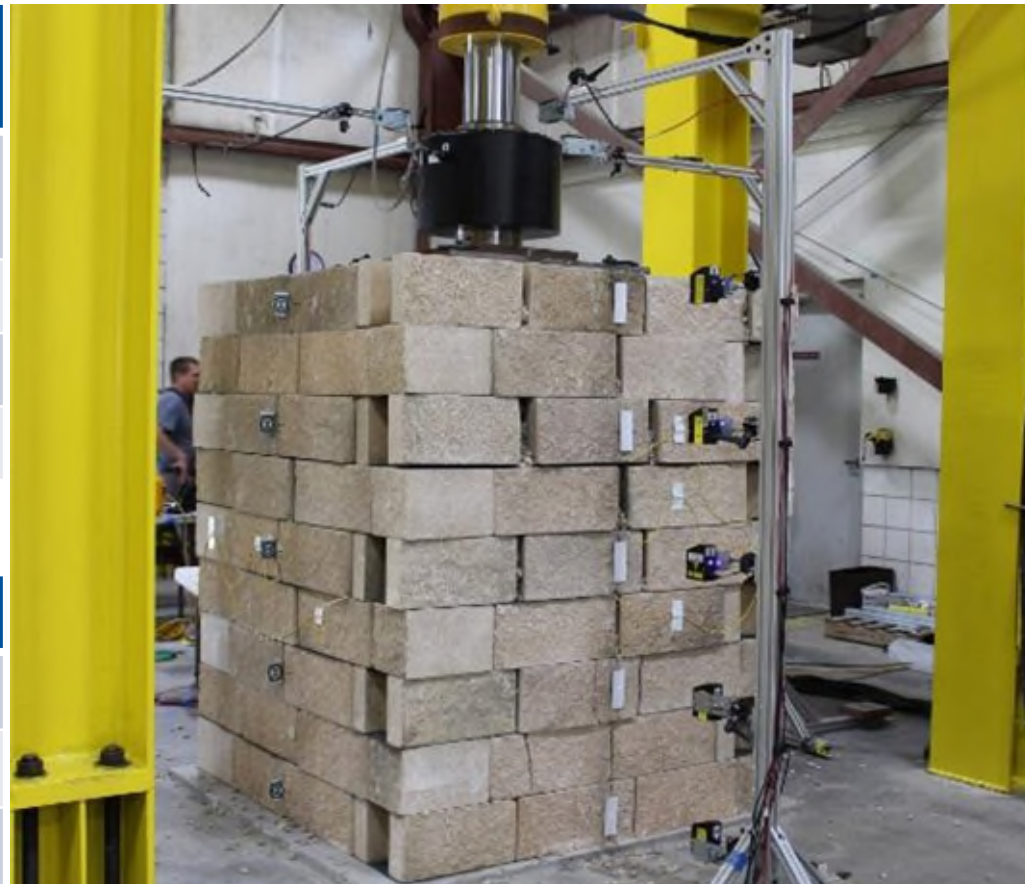
Photo of the failed pier after the test
