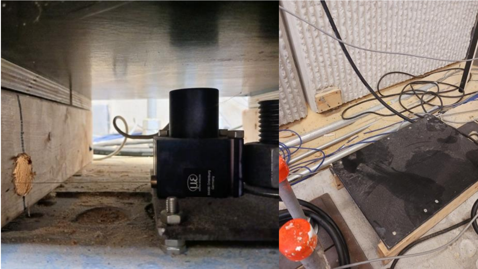
Draw-wire Sensors – Wall Displacement
