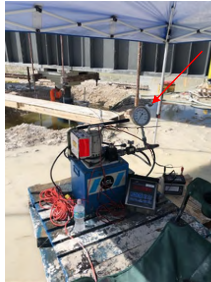
Construction for load test: Anchor Installation, Hydraulic Jack & Load Cell, load test.
