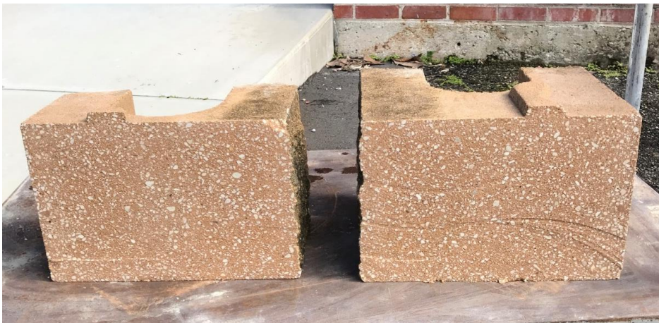
Vertical straight face blocks after being wet cut
