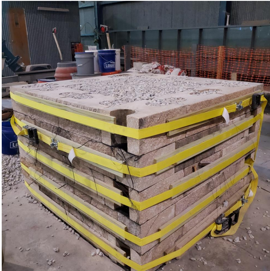
GRS test pier constructed to limited height with five courses
