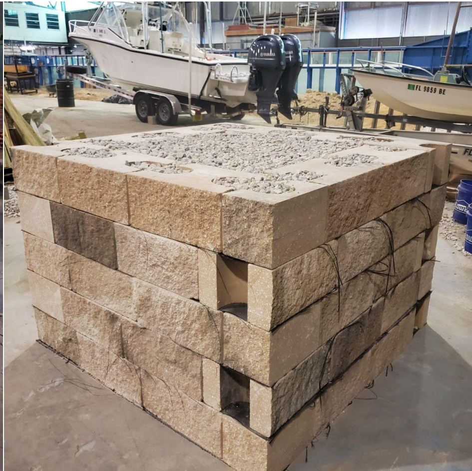
GRS test pier constructed to limited height with five courses
