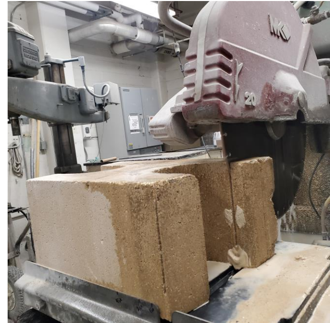
Cutting of blocks (Wet saw)
