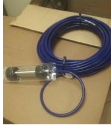
Vibration wire piezometers, readout, and datalogger
