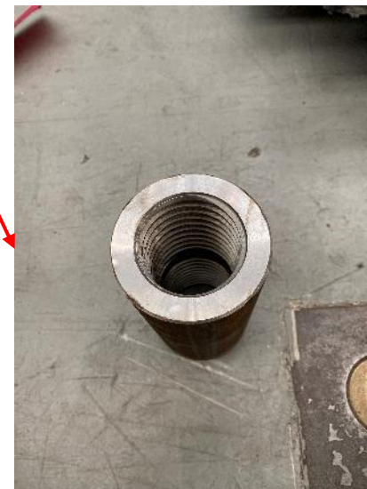
Coupler for #18 Grade 80 Threaded Rebars
