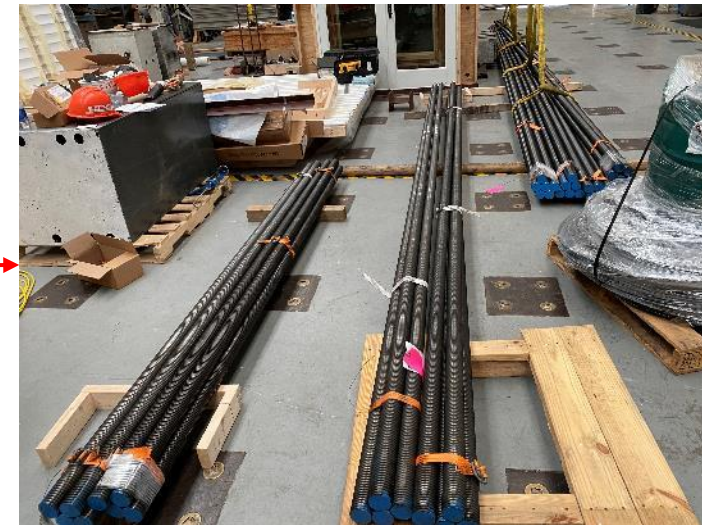
#18 Grade 80 Threaded Rebars, From left to right: 10 ft, 20 ft, 36 ft
