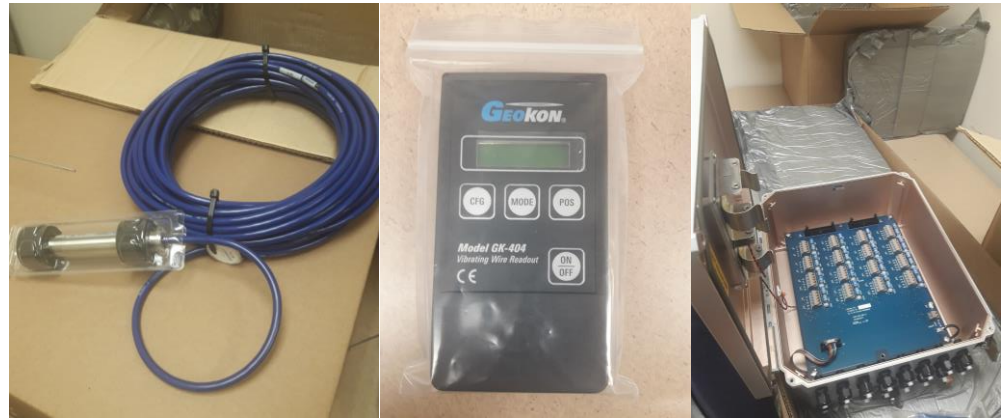
Vibration wire piezometers, readout, and datalogger
