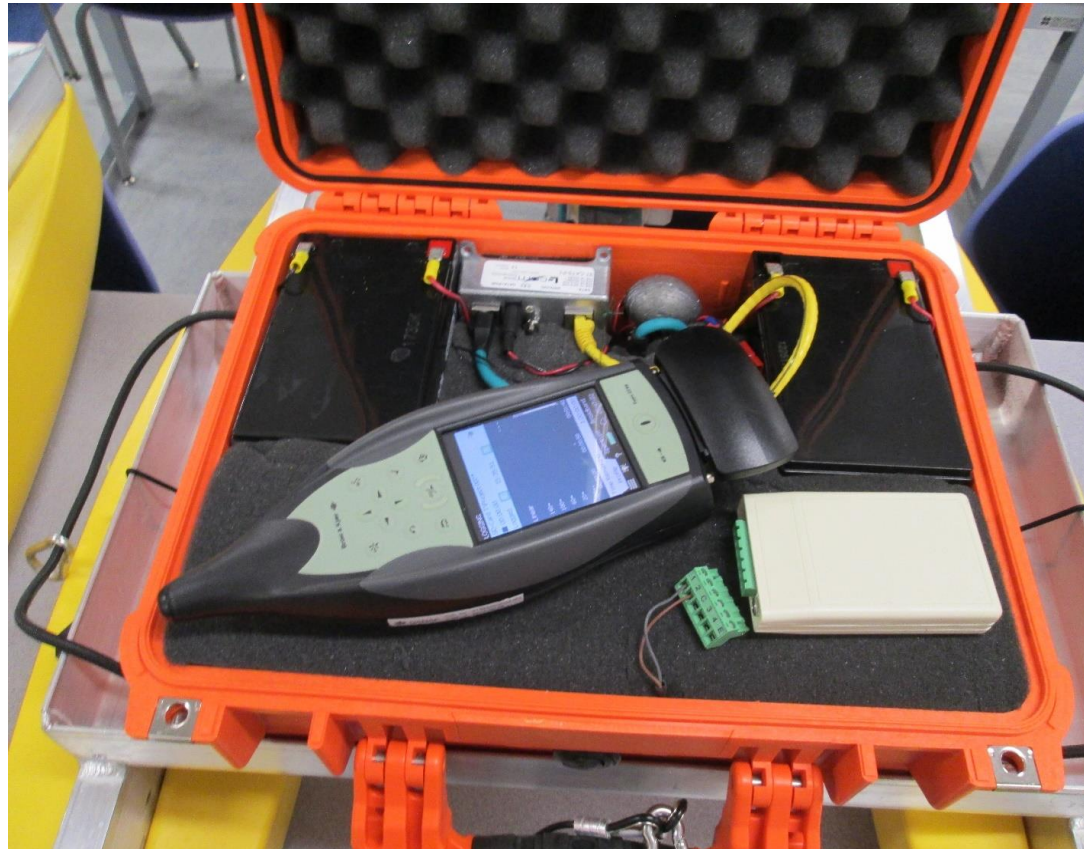
Data loggers, batteries, power converters, etc.
