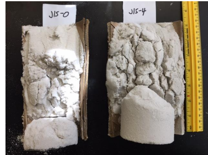
Typical Percolation Results in 50/70 Ottawa Sand
