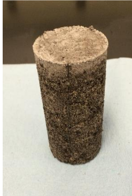
Fully Calcified OC Specimen Examples (post MICP treatment) Showing (a) 50/70 Ottawa Sand with 10% OC; (b) 50/70 Ottawa Sand with 30% OC; (c) 50% OC with 50% SDS; and (d) 50% OC with 80% SDS
