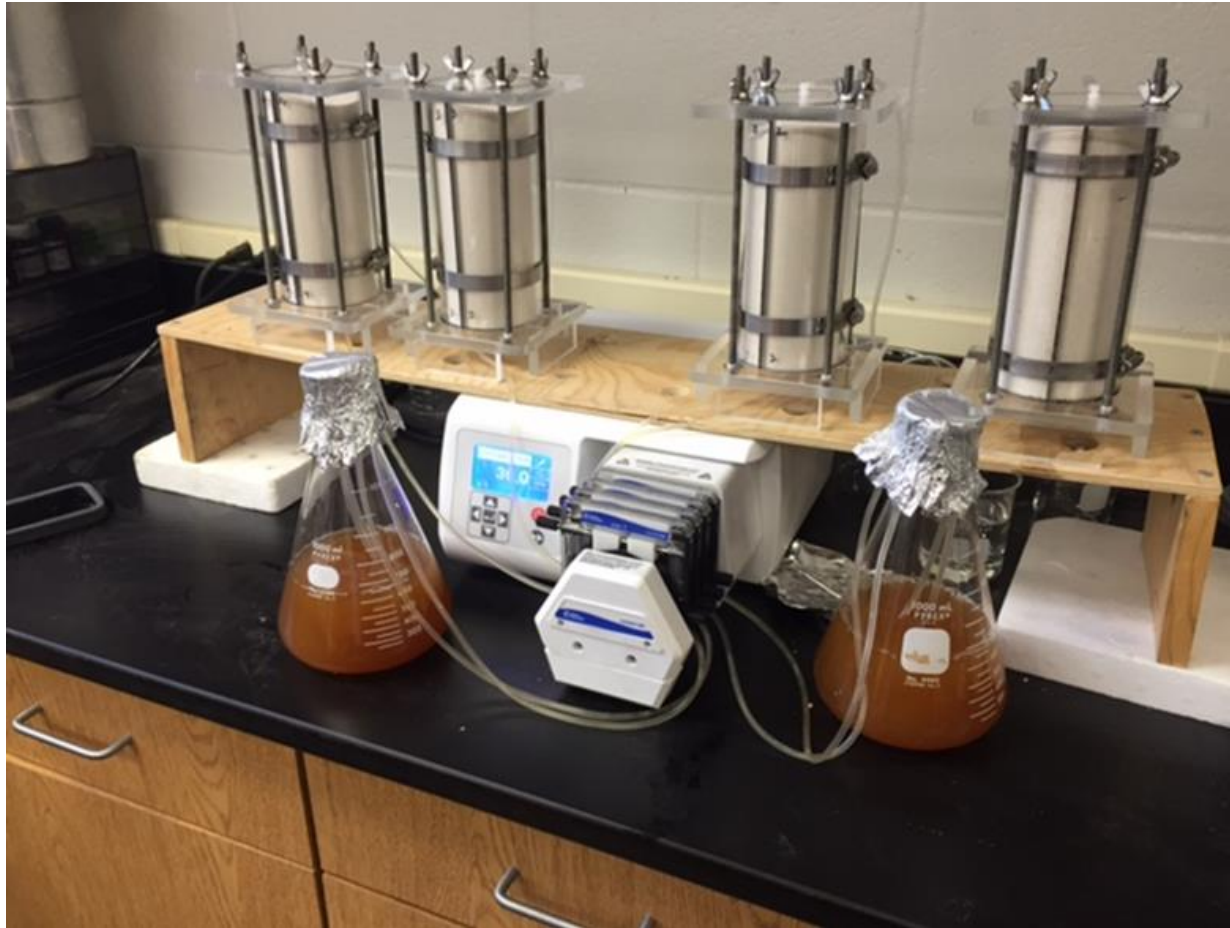
Soil Percolation Setup
