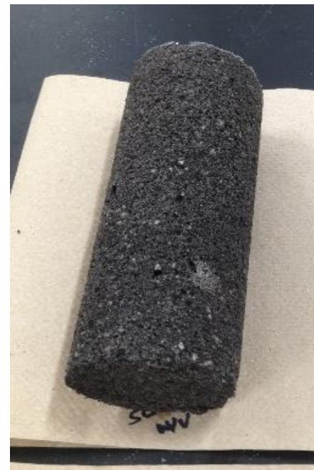
Fully Calcified OC Specimen Examples (post MICP treatment) Showing (a) 50/70 Ottawa Sand with 10% OC; (b) 50/70 Ottawa Sand with 30% OC; (c) 50% OC with 50% SDS; and (d) 50% OC with 80% SDS
