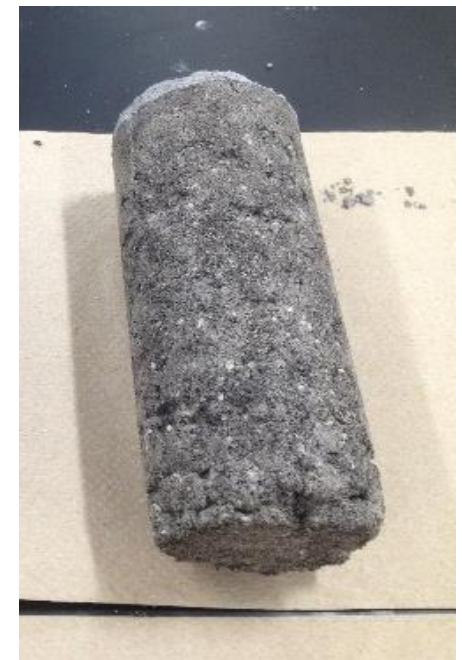
Fully Calcified OC Specimen Examples (post MICP treatment) Showing (a) 50/70 Ottawa Sand with 10% OC; (b) 50/70 Ottawa Sand with 30% OC; (c) 50% OC with 50% SDS; and (d) 50% OC with 80% SDS
