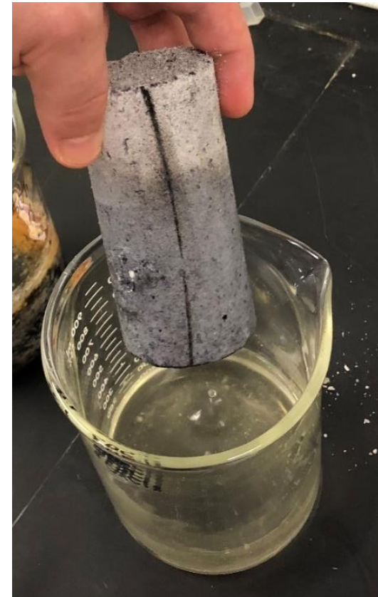
50% OC, 30% SDS, & 2.5M CaCl after 3 Weeks
