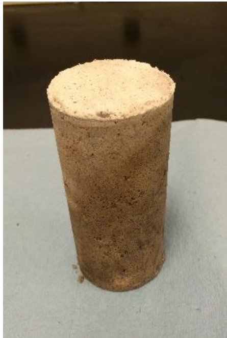
Fully Calcified OC Specimen Examples (post MICP treatment) Showing (a) 50/70 Ottawa Sand with 10% OC; (b) 50/70 Ottawa Sand with 30% OC; (c) 50% OC with 50% SDS; and (d) 50% OC with 80% SDS
