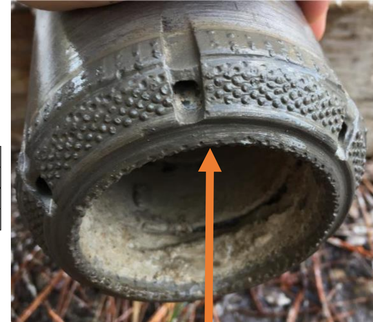
Missing cutting teeth
