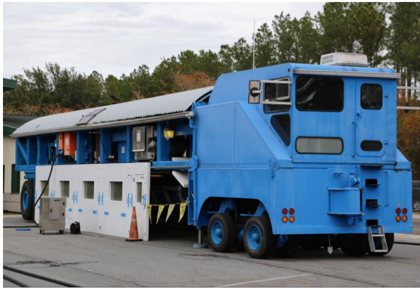
Figure 4. FDOT’s HVS Mark 4 utilized in fatigue performance evaluation
