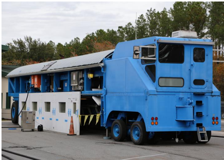
Figure 3. HVS used for accelerated loading in FDOT's APT facility
