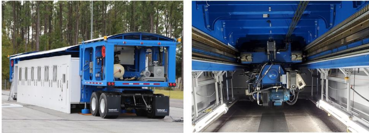
6 7 8 Figure 4. FDOT's HVS Equipment in the APT Facility 9
