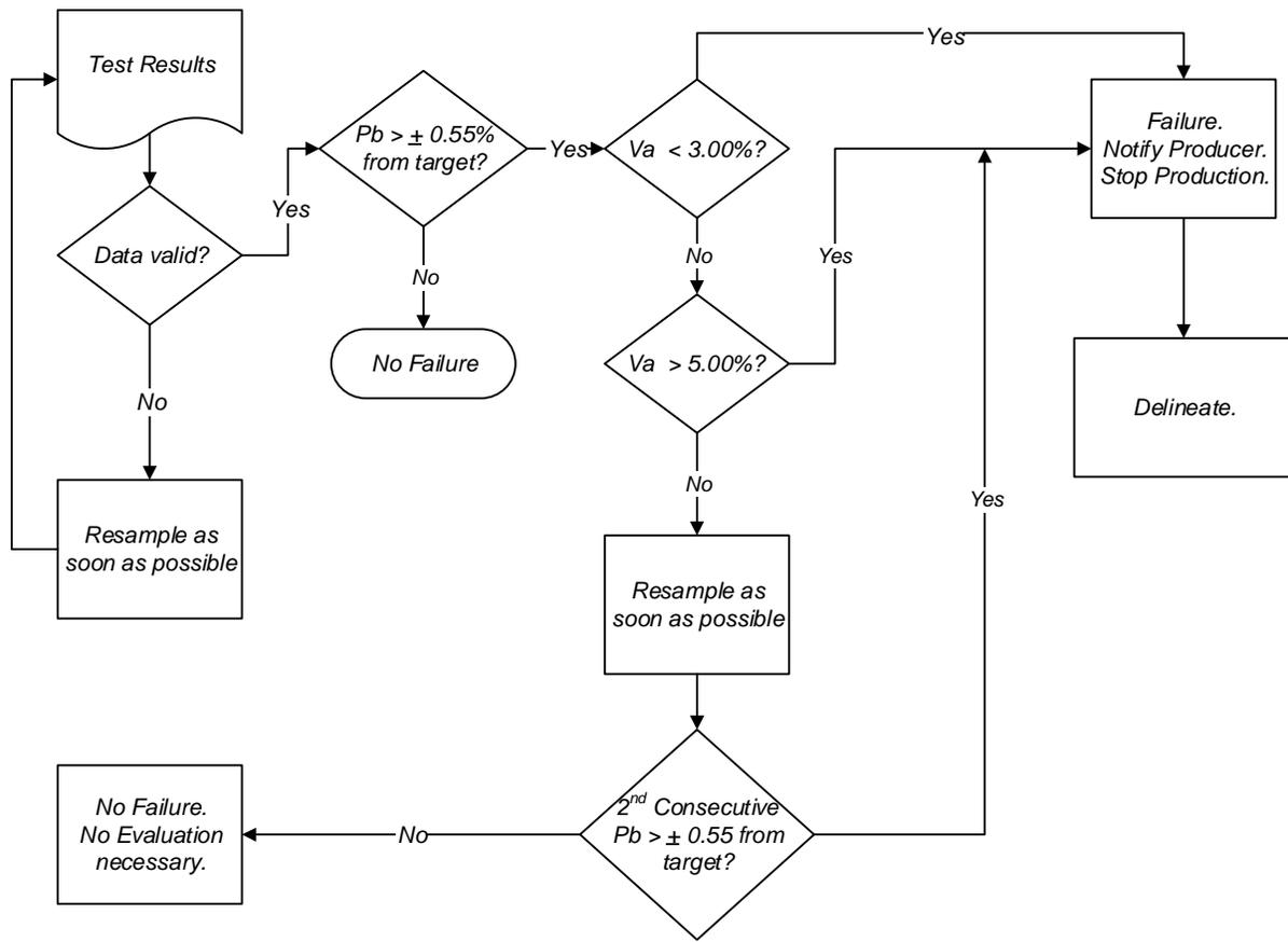
**Figure 3 Asphalt Binder Content (P<sub>b</sub>) – Dense Mixes**
