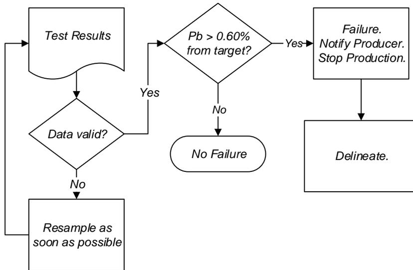
**Figure 4 FC-5 Asphalt Binder Content (P<sub>b</sub>)**
