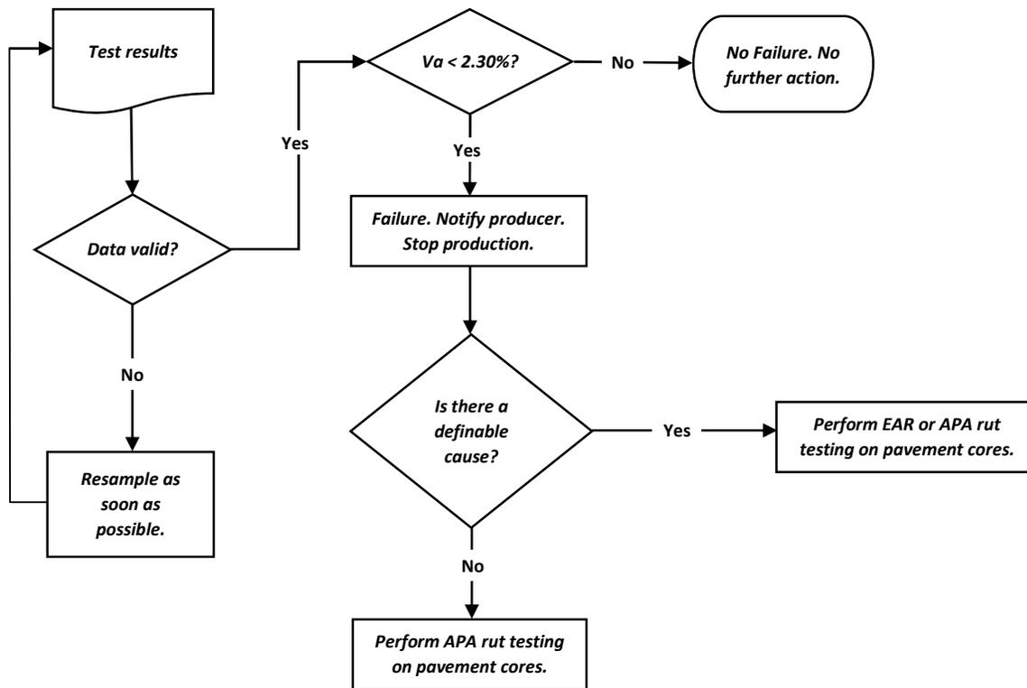
**Figure 1 Low Air Voids at the Asphalt Plant – Dense Mixes**
