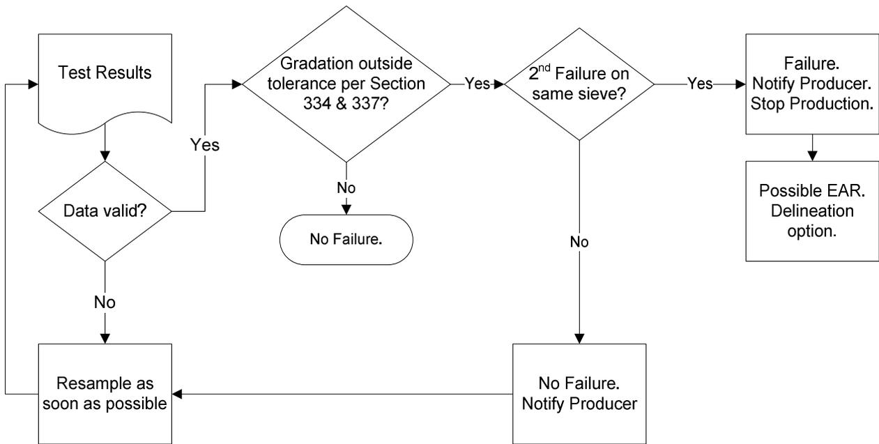
**Figure 6 Gradation Failures**
