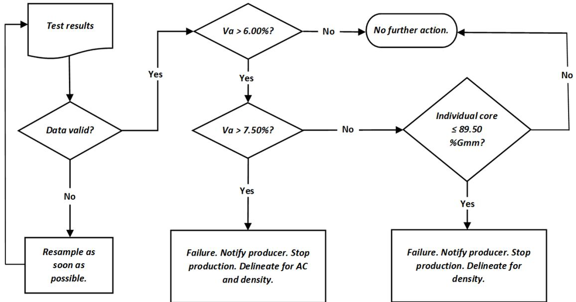
**Figure 2 High Air Voids at the Asphalt Plant – Dense Mixes**
