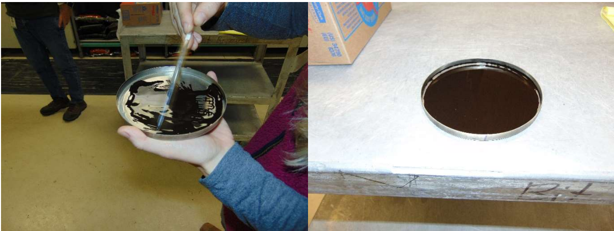
Figure 1 – Spreading the Emulsion in the PAV Pan
