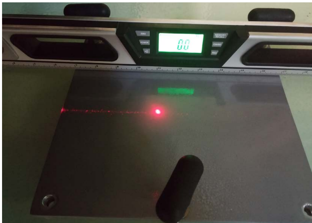
Figure 5. MPSV Calibration for CS and G (Detail of Calibration Plate Placed Under Rear Laser Sensor)
