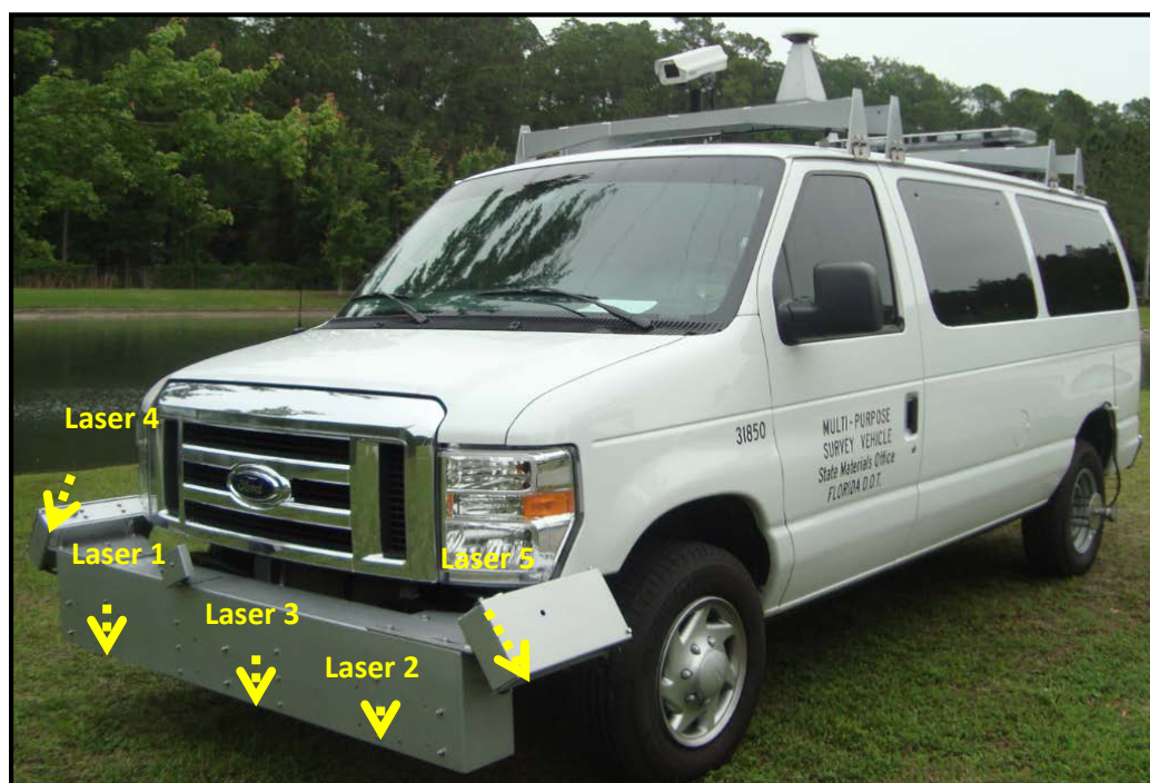
Figure 1. FDOT MPSV with 5 Laser Height Sensors Mounted in the Front Bumper
