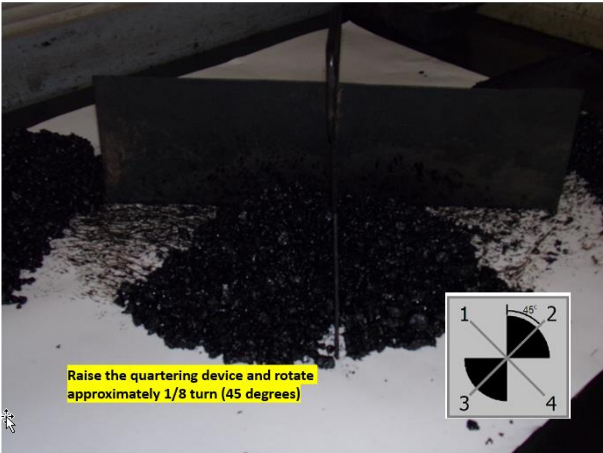
Figure 5. Raising and rotating the quartering device.
