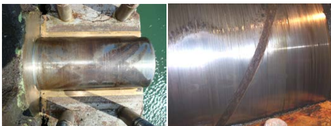
Figure 2.8.2.11.3.2.1-1 – Scored sheave shaft; while not visible in this photo, shaft has bronze imbedded in the surface, indicating “severe” wear on bushing
