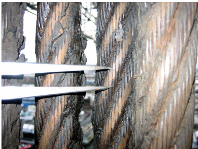
Figure 2.8.2.11.3.1-1 – Flattened areas on the wire rope indicate abrasive wear
