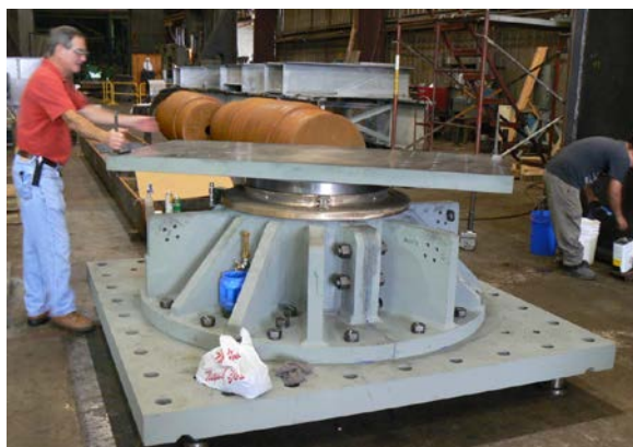
Figure 2.8.2.11.2.1.1-1 – A new spherical bronze center bearing for a swing bridge
