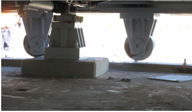
Figure 2.8.2.11.2.2.1-1 – Close-up of balance wheel with excessive clearance
