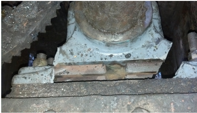
Figure 2.8.2.3.1.1-2 – Pillow block with complete failure in the fillet area
