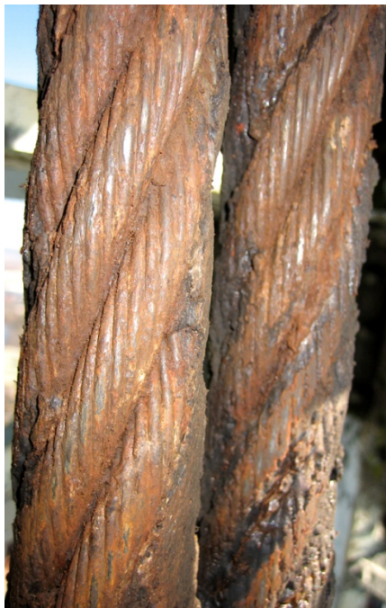
Figure 2.8.2.11.3.1-2 – Heavily corroded wire ropes; ropes with deterioration from corrosion should be evaluated for removal from service
