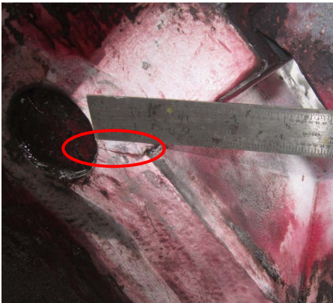
Figure 2.8.2.11.1.2.1-1 – Longitudinal crack in track girder tread plate
