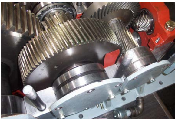
Figure 2.8.2.2.2-1 – Spiral bevel/helical gear, right angle speed reducer
