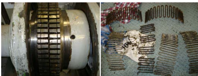
Figure 2.8.2.4.2.2.6-1 – Interior of a well-lubricated grid coupling; note broken grids
