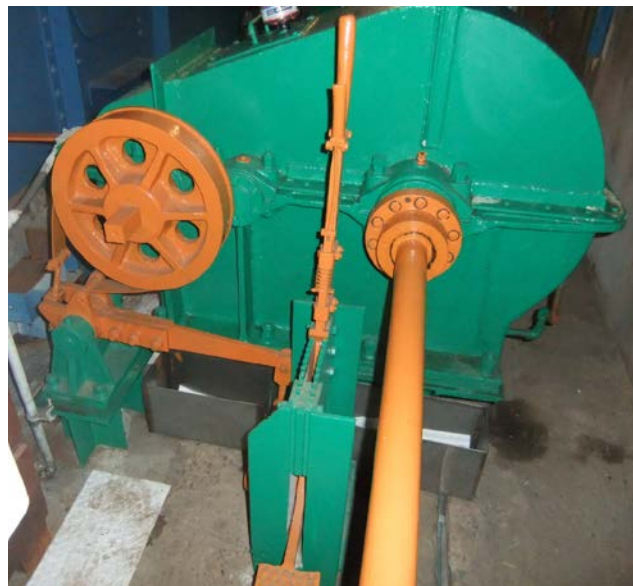
Figure 2.8.2.8.3-1 – Manual span brake, inoperable due to corrosion and excessive paint
