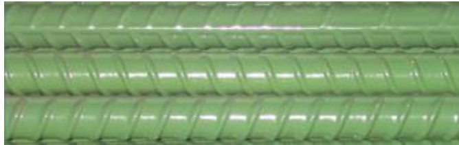
Figure 7.2 Epoxy Coated Reinforcement
