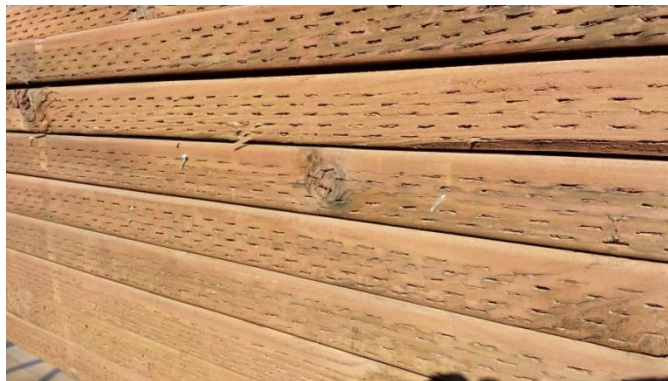
Figure 7.49 Typical Pressure Treated Markings (Courtesy of Michael B. Johnson)
