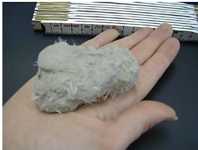
Figure 7.6 Concrete Fiber Reinforcement
