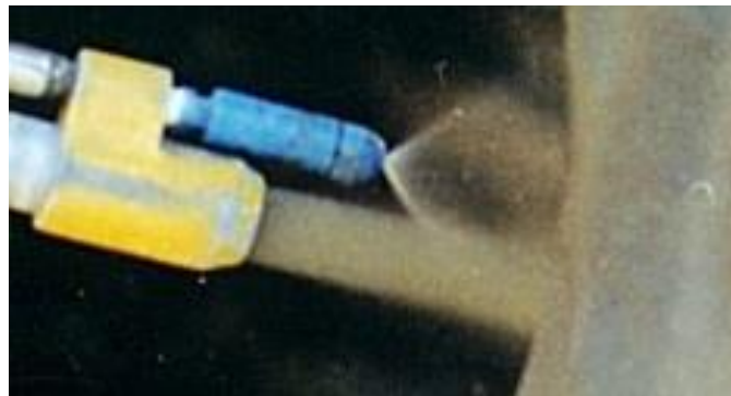
Figure 5.61 Mix Water Added at Nozzle
