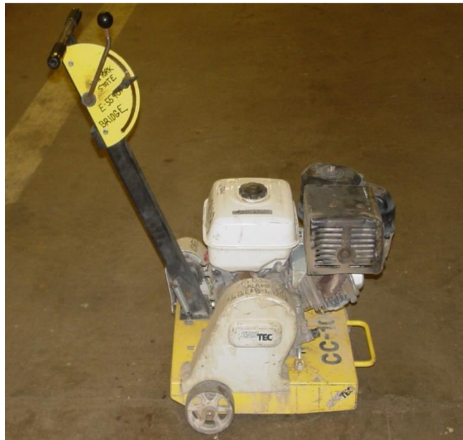
Figure 5.74 Crack Router for Preparing Horizontal Cracks
