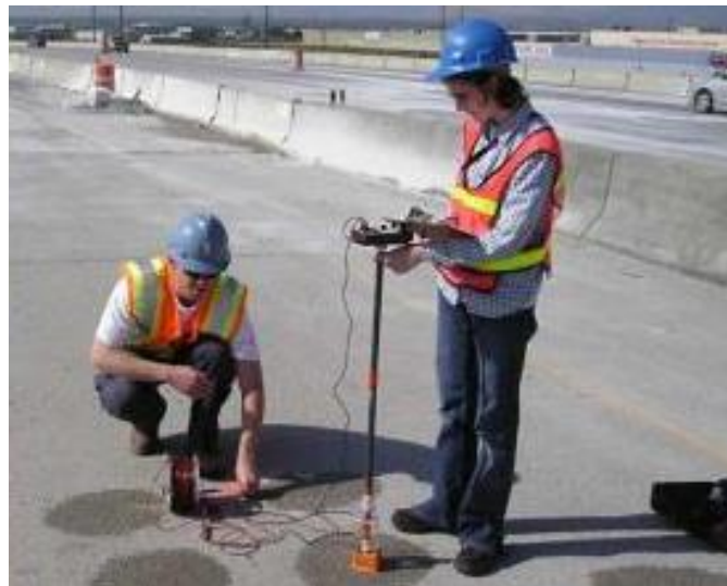
Figure 5.15 Example of Half-Cell Potential Test
