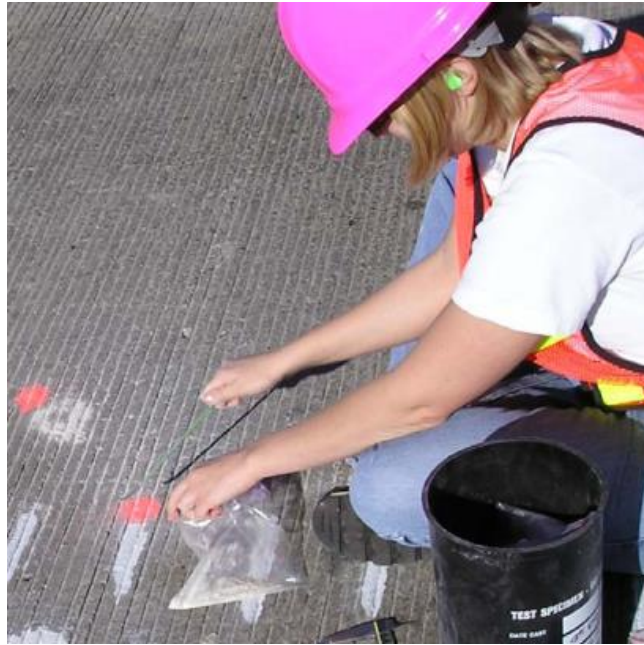
Figure 5.33 Chloride Profile Sample Collection
