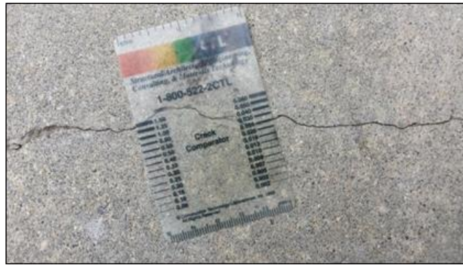
Figure 5.12 Crack Comparator for Determining Crack Width
