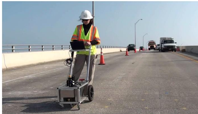
Figure 5.23 USW on Bridge Deck
