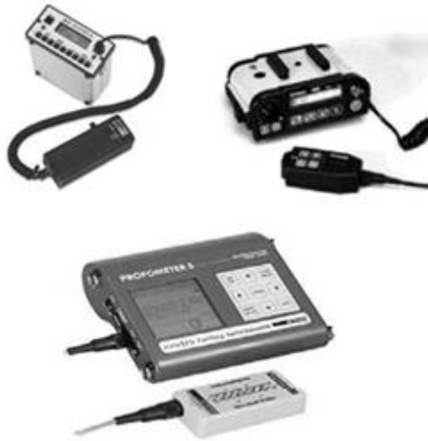
Figure 5.17 Examples of Pachometer Equipment
