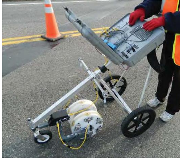
Figure 5.20 Impact Echo Testing
