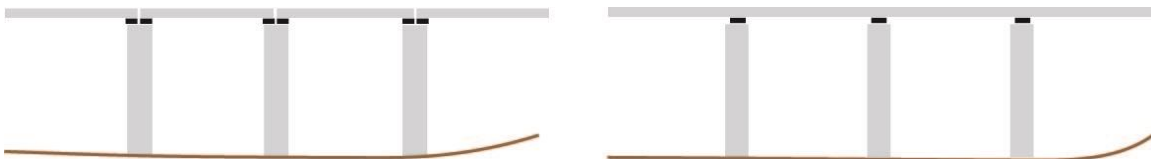
Figure 4.24 Structurally Non-Redundant Bridge vs. Structurally Redundant Bridge
