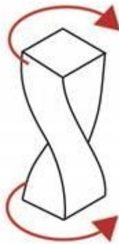
Figure 4.12 Torsion Forces Tend to Twist or Rotate the Member along the Longitudinal Axis
