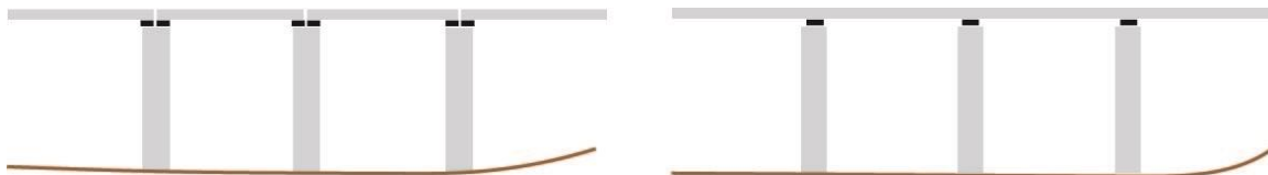
Figure 4.24 Structurally Non-Redundant Bridge vs. Structurally Redundant Bridge
