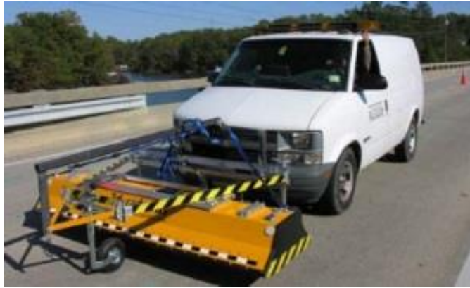
Figure 20.4 Van Mounted GPR
