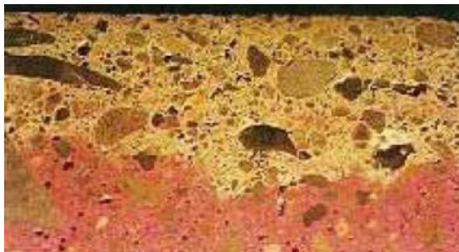
Figure 20.11 Phenolphthalein Reveals Noncarbonated Areas
