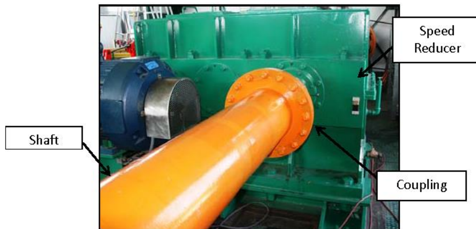
Figure 17.21 Speed Reducer (Closed Gearing), Shaft, and Coupling
