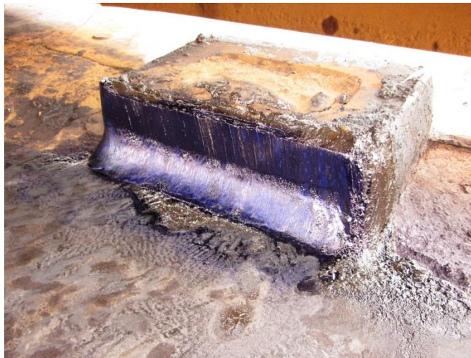
Figure 17.89 Excessive Wear of Tread Plate Tooth
