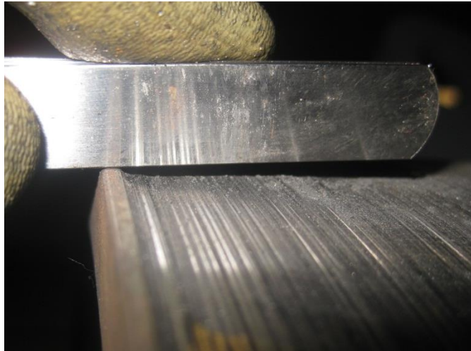
Figure 17.80 Close-up of Brakewheel Showing Significant Wear and Deep Grooves
