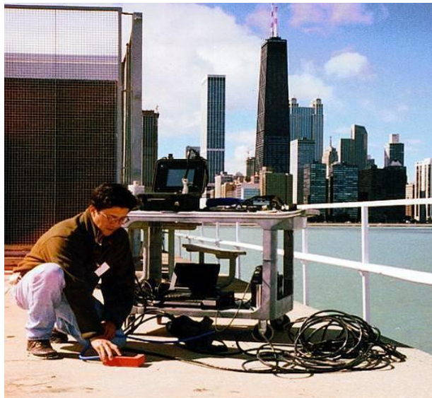
Figure 16.23 Ground Penetrating Radar Testing
