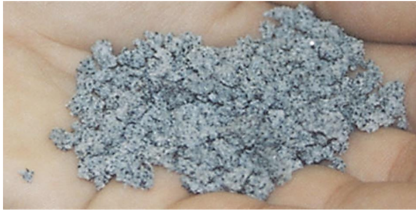
Figure 18.38 Sponge Media with Embedded Abrasive (Courtesy of SSPC)
