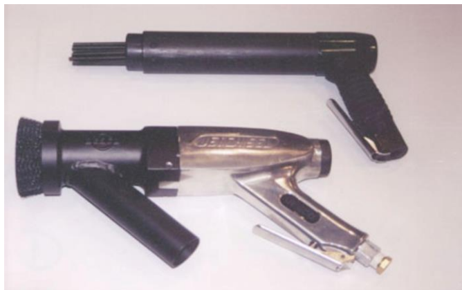
Figure 18.31 Needle Guns (Courtesy of SSPC)
