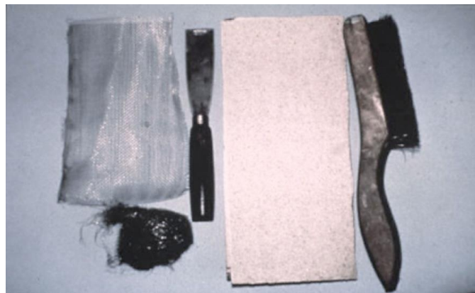
Figure 18.29 Various Hand Tools for Surface Preparation (SSPC)
