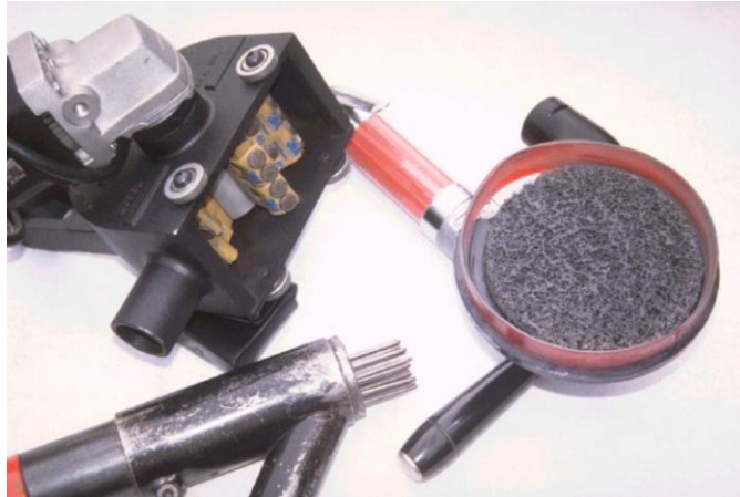
Figure 18.30 Common Power Tools for Surface Preparation (Courtesy of SSPC)
