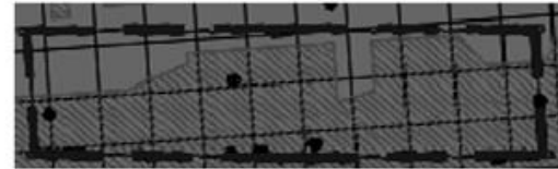
Delamination map (bottom) and rebar map (top) from GPR survey. Dark areas in top figure are delaminations which mask the rebar.
