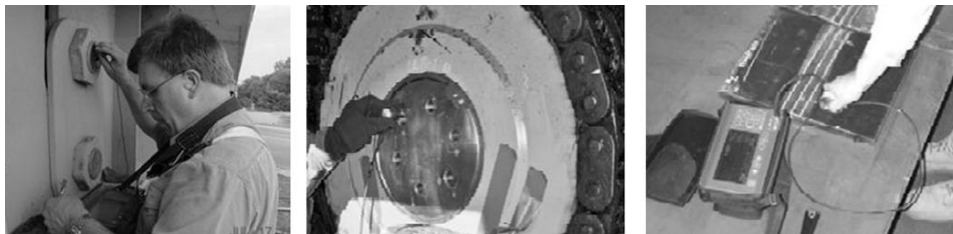
Figure B.19 UT Inspection of Bridge Hanger Pins (left), Bogie Shaft (middle), Sample CJP Weld (right)
